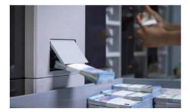
The BPS C5 also has an optional bander, the Bander Delivery Module (BDM) which automatically straps 100 notes of the denomination of your choice along with the information about that deposit, printed in real time, right on the strap. The BDM utilizes two grippers which alternate between stacking and strapping the notes to maintain an uninterrupted process.
